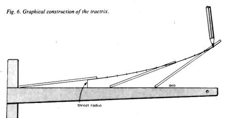
Using a straight edge of length equal to the final mouth radius, the tractrix curve is constructed of a series of tangents, length not greater than  $\frac{1}{10}$  the mouth radius, starting at the throat.
