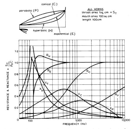
Fig. 1. Acoustical resistance and reactance against frequency at the throats of a series of infinite horns of different contour.
