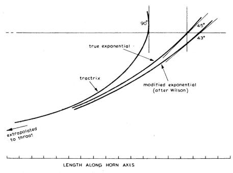
Fig. 5. Comparison of the exponential and tractrix contours.
