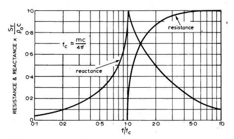
Fig. 3. Acoustical resistance and reactance of an exponential horn.
